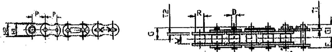
**10B-1** Roller chain made to ISO R606 is **5/8"** or **15.875 mm** pitch it is available in single strand **10B-1** duplex **10B-2** and triplex **10B-3**. It is possible to have the chain up to 6 strands wide.
